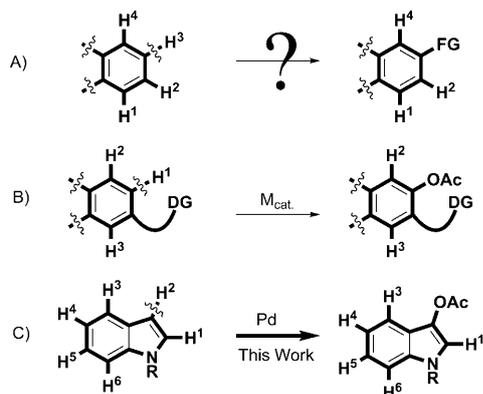
Scheme 1. Selectivities of direct C–H functionalizations of arenes: A) without and B) with a directing group as well as C) the approach used herein. FG=functional group; DG=directing group; the wavy lines highlight the chemical bonds involved in C–H activation process and represent the neglected structures in the molecules.
