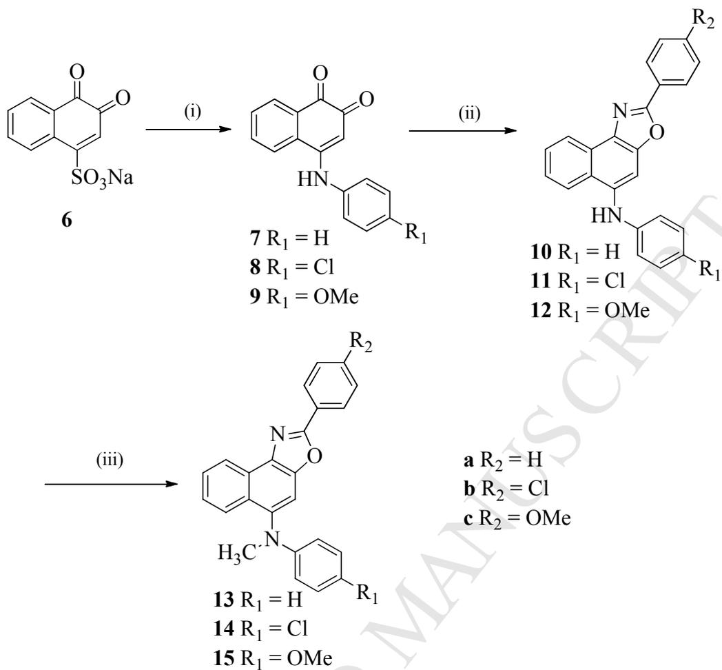
**Scheme 1:** Reagents and conditions: (i) substituted aniline,  $\text{H}_2\text{O}$ , rt, 20 min; (ii) substituted aldehyde,  $\text{NH}_4\text{OAc}$ ,  $\text{AcOH}$ ,  $150^\circ\text{C}$ , 2.5h (iii)  $\text{MeI}$ ,  $\text{NaH}$ , dry  $\text{DMF}$ , 10 min.
