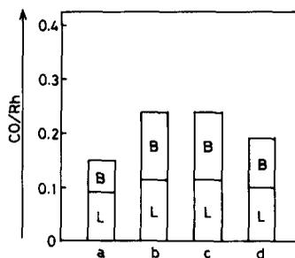
FIG. 4. Quantities of adsorbed CO species on Rh/Al<sub>2</sub>O<sub>3</sub> in competitive adsorption with H<sub>2</sub> at 473 K (CO/H<sub>2</sub>, 200/400 (Torr)). (a) 10 s; (b) 3-30 min; (c) 1 h; (d) after evacuation at 473 K for 1 h.
