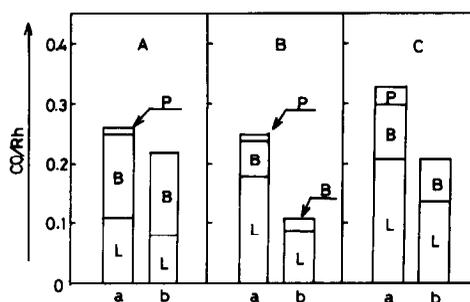
FIG. 2. Intensities of IR spectra of CO adsorbed on Rh catalysts at 473 K. (A) Rh/SiO<sub>2</sub>; (B) Rh/Al<sub>2</sub>O<sub>3</sub>; (C) Rh/TiO<sub>2</sub>. (a) CO, 200 Torr; (b) after evacuation at 473 K for 1 h.
