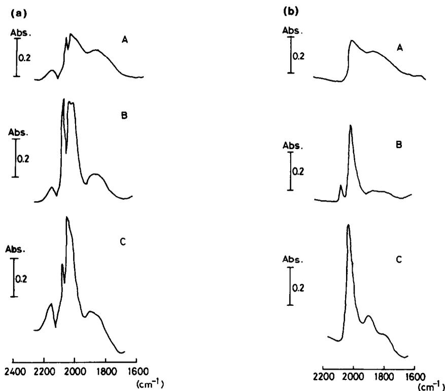
FIG. 1. (a) IR spectra of adsorbed CO at 473 K. (A) Rh/SiO<sub>2</sub>; (B) Rh/Al<sub>2</sub>O<sub>3</sub>; (C) Rh/TiO<sub>2</sub>.  $P_{\text{CO}} = 200$  Torr. (b) IR spectra of irreversibly adsorbed CO at 473 K. (A) Rh/SiO<sub>2</sub>; (B) Rh/Al<sub>2</sub>O<sub>3</sub>; (C) Rh/TiO<sub>2</sub>.
