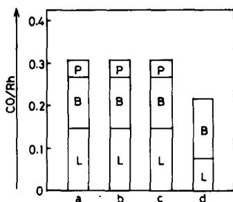
FIG. 3. Quantities of adsorbed CO species on Rh/SiO<sub>2</sub> in competitive adsorption with H<sub>2</sub> at 473 K (CO/H<sub>2</sub>, 200/400 (Torr)). (a) 10 s; (b) 3-30 min; (c) 1 h; (d) after evacuation at 473 K for 1 h.
