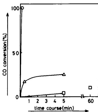
FIG. 5. Reactivity of irreversibly adsorbed CO with H<sub>2</sub> at 473 K. (□) Rh/SiO<sub>2</sub>; (△) Rh/Al<sub>2</sub>O<sub>3</sub>; (○) Rh/TiO<sub>2</sub>.
