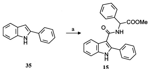
Scheme 6. (a) 1. ClCOOCCl<sub>3</sub>, pyridine, PhMe, r.t., 4 h; 2. (*R,S*)-methyl phenyl glycinate, Et<sub>3</sub>N, DMF, 0°C to r.t., overnight.
