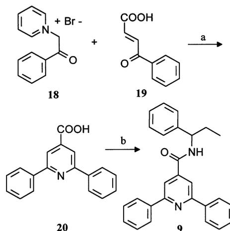
Scheme 1. (a) AcOH/Ac<sub>2</sub>O, (10:1), AcONH<sub>4</sub>, 100°C, 5 h; (b) DCC, HOBT, (±)-Ph(Et)CHNH<sub>2</sub>, THF/MeCN (1:1), r.t., 20 h.
