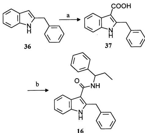
Scheme 7. (a) Triphosgene, pyridine, CH<sub>2</sub>Cl<sub>2</sub>, 3 h; then 5% NaHCO<sub>3</sub>, Et<sub>2</sub>O, overnight; (b) WSC, HOBT, (±)-Ph(Et)CHNH<sub>2</sub>, THF/CH<sub>3</sub>CN (1:1), r.t., overnight.
