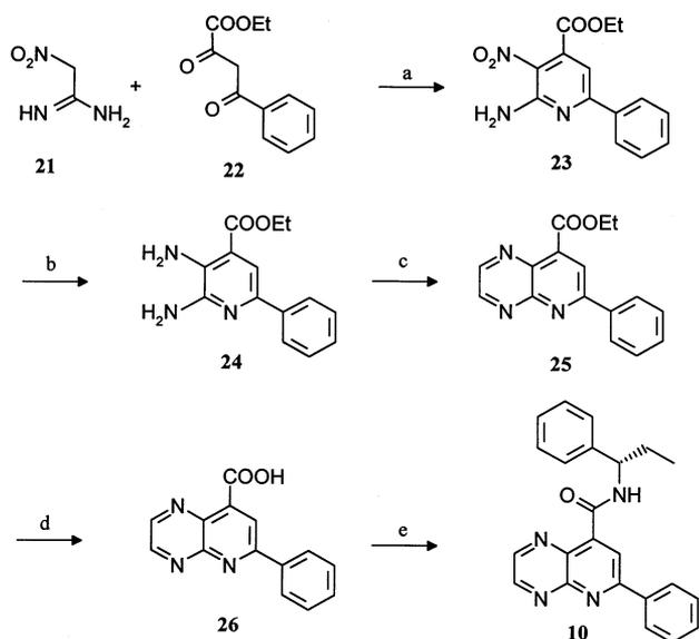
Scheme 2. (a) 95% EtOH, reflux, 20 h; (b) H<sub>2</sub>, 10% Pd/C, 95% EtOH/THF, (1:1), 22 h; (c) 2,3-dihydroxy-1,4-dioxane, 95% EtOH, 30 h; (d) KOH, EtOH/H<sub>2</sub>O (1:1), reflux, 3 h; then 1 N HCl; (e) DCC, HOBT, (S)-(-)-Ph(Et)CHNH<sub>2</sub>, THF/MeCN (1:1), r.t., 15 h.
