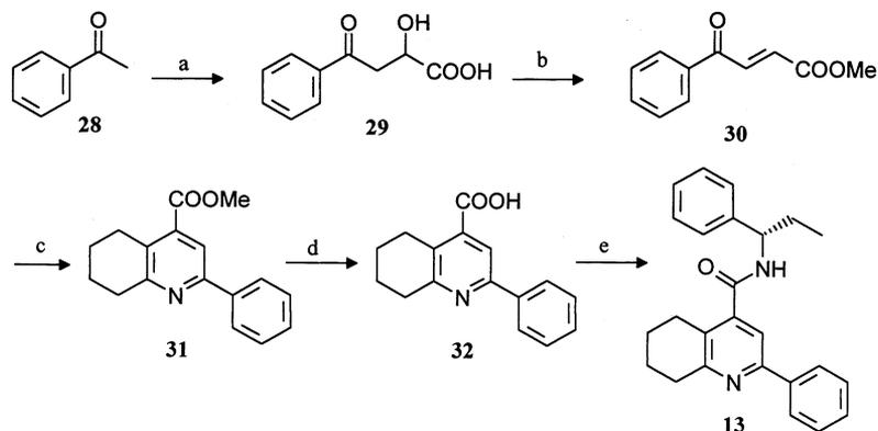
Scheme 4. (a) Glyoxylic acid, NaOH, MeOH/H<sub>2</sub>O (1:1), r.t., 24 h; (b) 1. NaHCO<sub>3</sub>, MeI, DMF, 18 h; 2. PTSA, PhMe, reflux, 1 h; (c) cyclohexanone, AcONH<sub>4</sub>, PhMe, reflux, 4 h; (d) NaOH, 95% EtOH, overnight; (e) DCC, HOBT, (*S*)-(-)-Ph(Et)CHNH<sub>2</sub>, THF/MeCN (1:1), r.t., 16 h.
