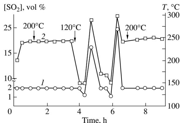
**Fig. 3.** Plots of the (1)  $SO_2$  concentration and (2) reaction temperature vs. reaction time at an  $H_2S$  concentration in the initial gas mixture of 2 vol %, an  $O_2/H_2S$  ratio of 5, and a contact time of 0.2 s. The temperature of the initial gas mixture changed during the reaction.
