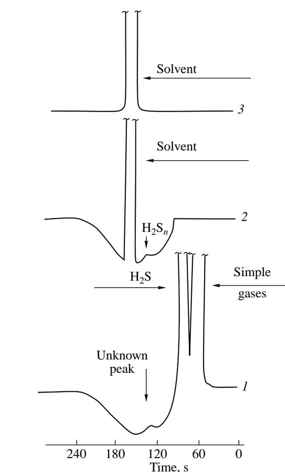
**Fig. 5.** Chromatograms of (1) the reaction gas mixture, (2) hydrogen polysulfide extracted with diethyl ether, and (3) solvent.
