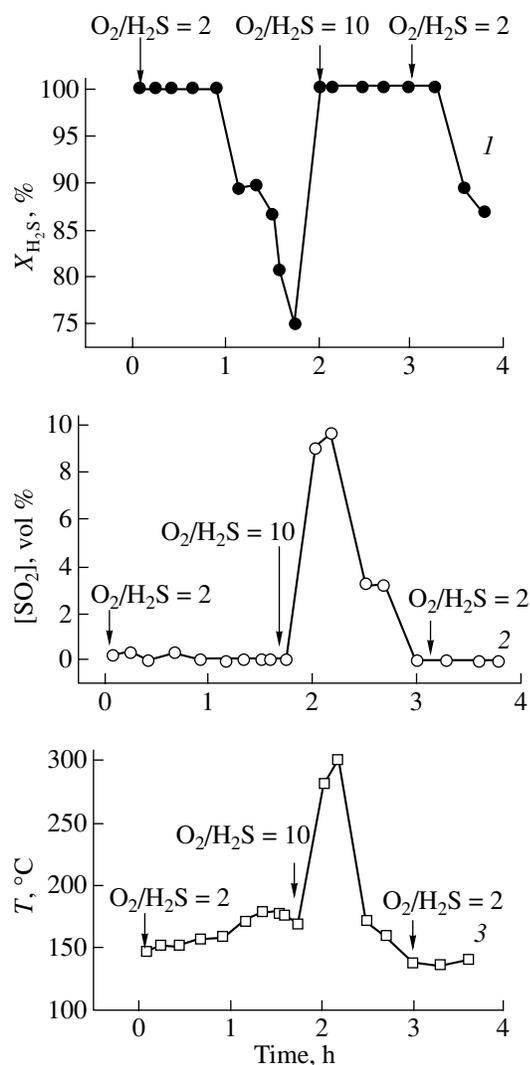
**Fig. 4.** Plots of the (1)  $H_2S$  conversion ( $X_{H_2S}$ ), (2)  $SO_2$  concentration, and (3) reaction temperature vs. reaction time at an  $H_2S$  concentration in the initial gas mixture of 2 vol %, a temperature of the initial gas mixture of 145°C, and a contact time of 0.2 s. The  $O_2/H_2S$  molar ratio changed during the reaction.
