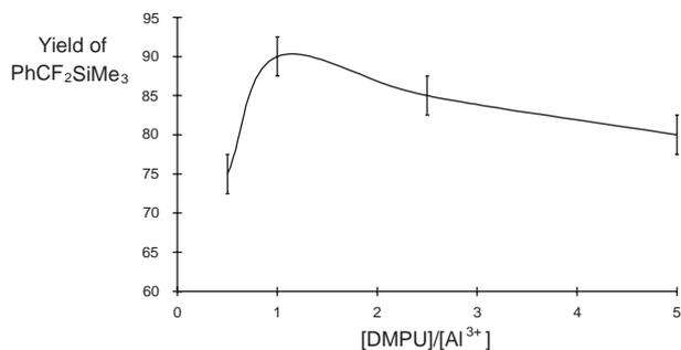
**Figure 2** Yield of  $\text{PhCF}_2\text{TMS}$  Depending on the ratio  $[\text{DMPU}]/[\text{Al}^{3+}]$
