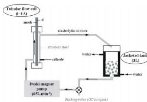
**Figure 3** Tubular Flow Cell
