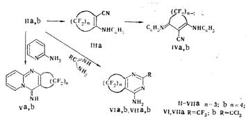
The IR spectra of III and IV contain vibrations at 3140-3270 (NH) and 2225-2235 cm<sup>-1</sup> (CN), as well as frequencies of C=N bonds at 1650-1660 cm<sup>-1</sup>. Vibrations at 3320-3400 (NH) and 1635-1640 cm<sup>-1</sup> (C=N) are observed in the IR spectra of pyrimidines Va,b.
