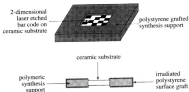
Figure 1. Illustration of the laser optical synthesis chip (LOSC), viewed from the top (top) and in cross-section (bottom). The size of the LOSC is 10 × 10 × 2 mm.
