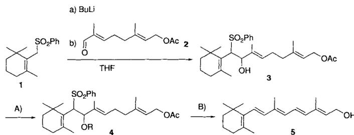
Scheme 1. Stepwise synthesis of vitamin A (5). A) Dihydropyran (R = tetrahydropyranyl), ethylvinyl ether/*p*-toluenesulfonic acid (R = 1-ethoxyethyl) or (MeO)<sub>2</sub>CH<sub>2</sub>/P<sub>2</sub>O<sub>5</sub> (R = MOM) in CH<sub>2</sub>Cl<sub>2</sub> or neat. B) *t*BuOK or MeOK in cyclohexane.
