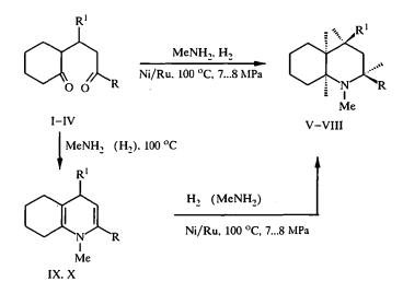
I, V, IX R = R<sup>1</sup> = Ph; II, VI R = Ph, R<sup>1</sup> = C<sub>6</sub>H<sub>4</sub>-OMe-*p*; III, VII R = C<sub>6</sub>H<sub>4</sub>-OMe-*p*, R<sup>1</sup> = Ph; IV, VIII, X R = Ph, R<sup>i</sup> = C<sub>6</sub>H<sub>4</sub>-Cl-*p*
