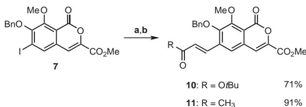
**Scheme 3** Reagents and conditions: a) *tert*-Butyl acrylate, Pd(OAc)<sub>2</sub>, PPh<sub>3</sub>, LiCl, Et<sub>3</sub>N, DMF, 85 °C, 8 h; b) 3-buten-2-one, Pd(OAc)<sub>2</sub>, *n*-Bu<sub>4</sub>NCl, NaHCO<sub>3</sub>, DMF, r.t., 72 h.
