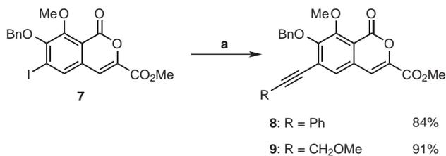
**Scheme 2** Reagents and conditions: a) R-C≡CH, Pd(OAc)<sub>2</sub>, PPh<sub>3</sub>, CuI, Et<sub>3</sub>N, DMF, r.t., 8 h.
