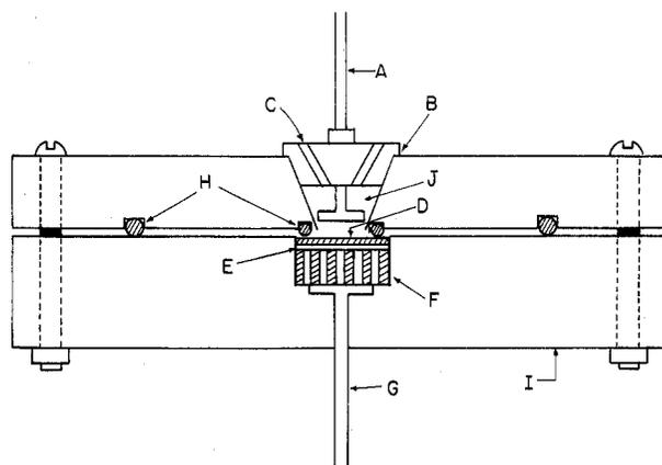
**Figure 1.** Reaction cell diagram: (A) mechanical stirrer; (B) Teflon plug; (C) sample injection ports; (D) dimethylsilicone rubber membrane supported on a polycarbonate filter; (E) stainless steel screen; (F) porous brass support; (G) tubing to the mass spectrometer; (H) Viton O-rings; (J) reaction compartment with a volume of approximately 0.5 mL.
