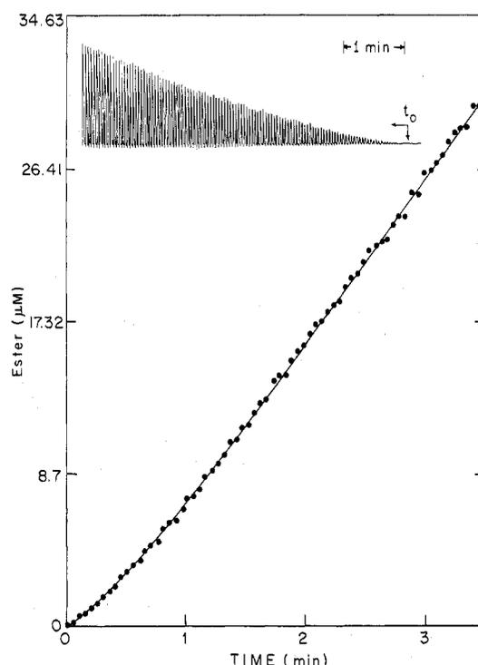
**Figure 3.** Mass spectrometer signal response during the enzymatic production of ethyl 2-furoate. Experimental conditions have been given in the text. The curve on the top is a tracing of the chart recording with the MS scanning the base peak ( $m/e = 112$ ). The solid curve was calculated from the best fit of eq 4 to the points.
