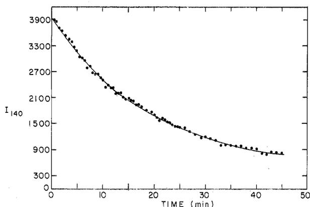
**Figure 4.** Permeation loss of ethyl 2-furoate through the membrane. The conditions have been given in the text; initial ester concentration was 20  $\mu\text{M}$ . The signal obtained from the molecular ion ( $m/e = 140$ ) is given in arbitrary units. The solid curve represents the best fit of a first-order decay curve through the experimental points.
