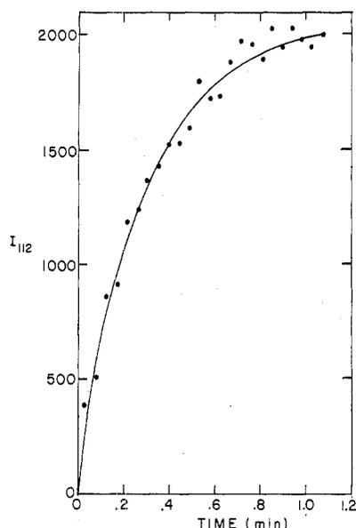
**Figure 2.** Mass spectrometer signal response after a single addition of ethyl 2-furoate. The signal magnitude obtained in the base peak ( $m/e = 112$ ) is given in arbitrary units. The line through the points was calculated from the best fit of eq 3 to the data. Ester concentration was  $15 \mu\text{M}$  and temperature was  $25^\circ\text{C}$ .
