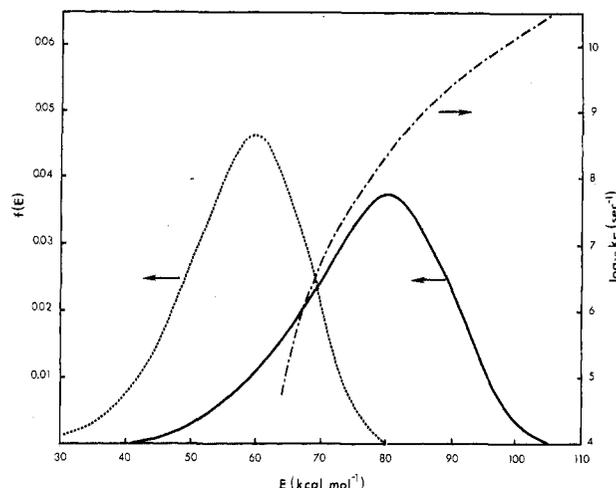
**Figure 5.** The value of  $k_E$  for cyclopropane isomerization to propylene ( $-\cdots-$ ), and examples of two statistical energy distribution functions:  $E^+ = 81$  kcal ( $\cdots$ ) and  $E^+ = 107$  kcal ( $-$ ).
