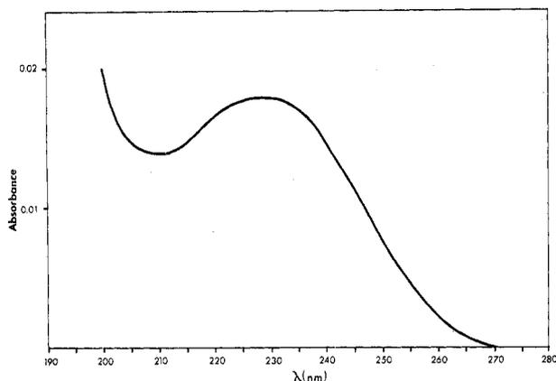
Figure 1. The gas-phase absorption spectrum of  $\sim 0.45$  torr of trimethylene sulfoxide in a 10-cm path length cell at 296 K.
