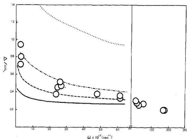
**Figure 3.** The propylene/cyclopropane ratio as a function of the collision rate of cyclopropane, 229-nm photolysis. The lines are calculated curves for  $E^+ = 99$  kcal ( $\cdots$ ),  $E^+ = 89$  kcal ( $-\cdots-$ );  $E^+ = 86$  kcal ( $-\cdot-\cdot-$ ), and  $E^+ = 81$  kcal ( $-$ ).
