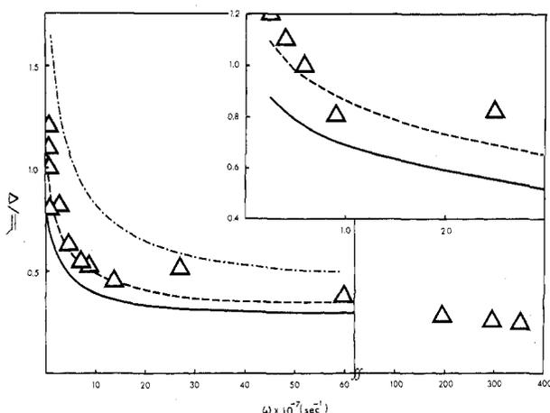
**Figure 4.** The propylene/cyclopropane ratio as a function of the collision rate of cyclopropane, 214-nm photolysis. The lines are calculated curves for  $E^+ = 99$  kcal ( $-\cdots-$ );  $E^+ = 93$  kcal ( $-\cdot-\cdot-$ ), and  $E^+ = 89$  kcal ( $-$ ).
