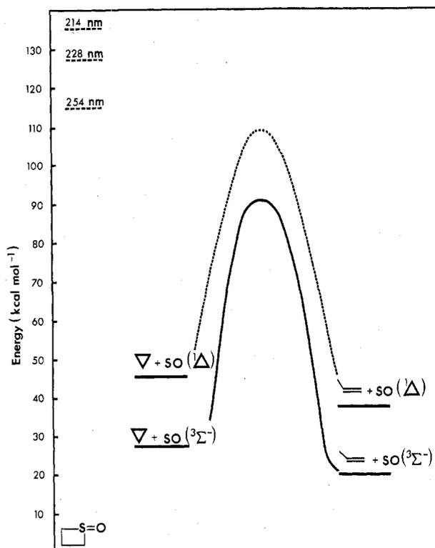
Figure 6. A schematic illustration of the energetics of the trimethylene sulfoxide system. Trimethylene sulfoxide is taken as the zero of energy, and the barrier is to indicate the magnitude of the critical energy for isomerization of cyclopropane to propylene.
