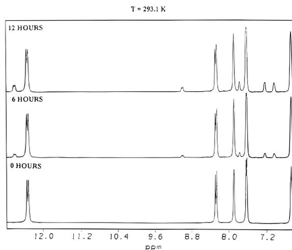
Figure 1. The 400 MHz  $^1\text{H}$  NMR spectrum of **3** as a function of time at 293.1 K.
