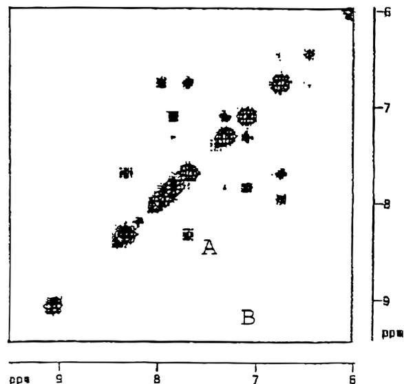
Figure 5. NOESY spectrum of a mixture of **3** and **4** in DMSO- $d_6$ . A: Cross-peak between the vinyl proton and the 4-H of the pyridine ring of **3**. B: Region where the expected cross-peak between the vinyl proton and the 4-H proton of the pyridine was not observed.
