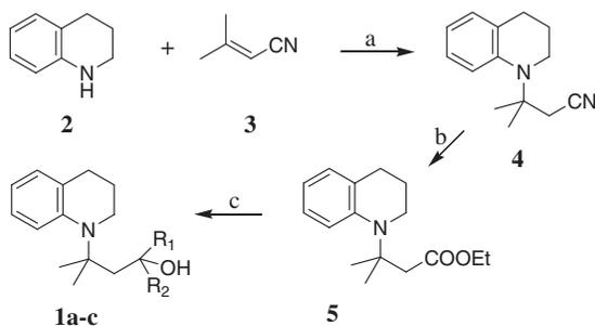
was readily synthesized in one step by the reaction of tetrahydroquinoline (**2**) with 3-methylcrotononitrile (**3**) in the presence of a catalytic amount of Triton B; **4** was successively converted to its ethyl ester **5**. The ethyl 3-(3,4-dihydroquinolin-1(2*H*)-yl)-3-methylbutanoate (**5**) was finally reacted with two equivalents of Grignard reagents to afford alcohols **1a–c**. The results are presented in Scheme 2 and Table 1 (Entries 1–3).
