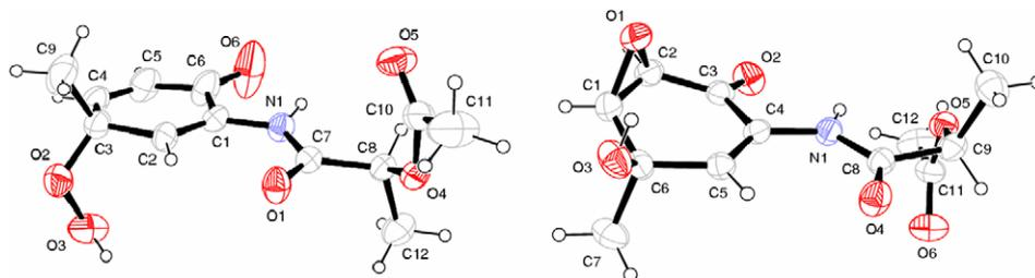
Figure 2. X-ray crystal structures of hydroperoxide **8a** (left) and epoxide **10b** (right).
