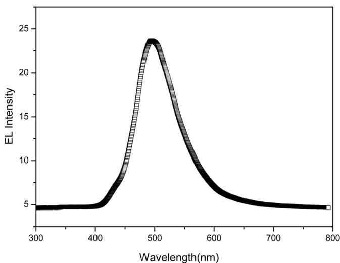
**FIGURE 3** EL spectrum of ITO/PEDOT:PSS(50 nm)/POTOSF(70 nm)/LiF(1 nm)/Al(200 nm) device at 20 mA/cm<sup>2</sup>.
