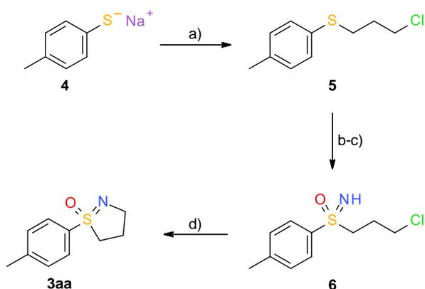
**Scheme 1.** Unexpected synthesis of cyclic sulfoximine **3aa** by Johnson and Janiga.<sup>[9]</sup> a) 1-bromo-3-chloropropane, dioxane, H<sub>2</sub>O, 86%; b) sodium periodate, H<sub>2</sub>O, 99%; c) NaN<sub>3</sub>, H<sub>2</sub>SO<sub>4</sub>, CHCl<sub>3</sub>, 89%; d) precipitate (insoluble in DCM) was dissolved in H<sub>2</sub>O and neutralized with aqueous NaOH, yield not reported.
