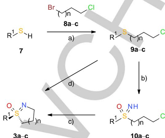
**Scheme 2.** Novel synthetic approach to cyclic sulfoximines **3**: a) NEt<sub>3</sub> (2 equiv), THF, RT; b) PhI(OAc)<sub>2</sub> (2.5 equiv), H<sub>2</sub>NCO<sub>2</sub>NH<sub>4</sub> (2–2.5 equiv), MeOH, RT; c) aqueous 0.1% NH<sub>3</sub>, 80 °C; d) PhI(OAc)<sub>2</sub> (2.5 equiv), H<sub>2</sub>NCO<sub>2</sub>NH<sub>4</sub> (2 equiv), MeOH, RT until full conversion of **9** into **10**, then stirring of the mixture in a closed vial at 80 °C; a: n = 1, b: n = 2, c: n = 3.
