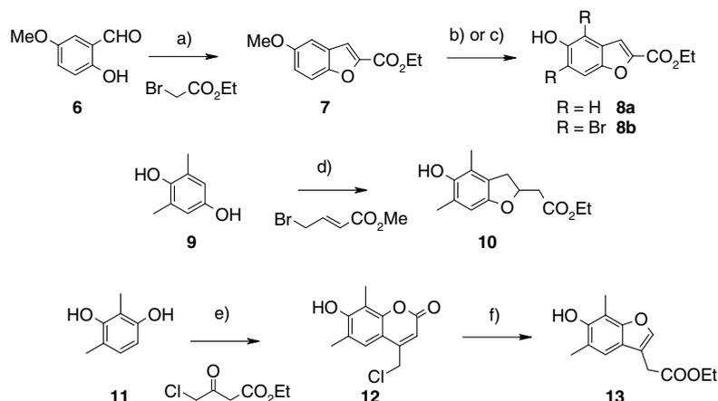
**Scheme 1.** Synthesis of benzofuran fragments. Reagents and conditions: (a)  $K_2CO_3$ , DMF, 80 °C (33%); (b)  $BBr_3$ , DCM, rt (39%); (c)  $i-BBr_3$ , DCM, rt (39%); ii— $Br_2$ , HOAc, 50 °C (21%); (d)  $i-ZnCl_2$  (1.7 equiv) *n*-heptane, reflux; ii—EtOH, concd  $H_2SO_4$ , reflux (6%); (e) concd  $H_2SO_4$ , rt (87%); (f)  $i-0.1$  N NaOH, reflux (69%); ii— $H_2SO_4$  (cat.), EtOH, reflux, 16 h (75%).
