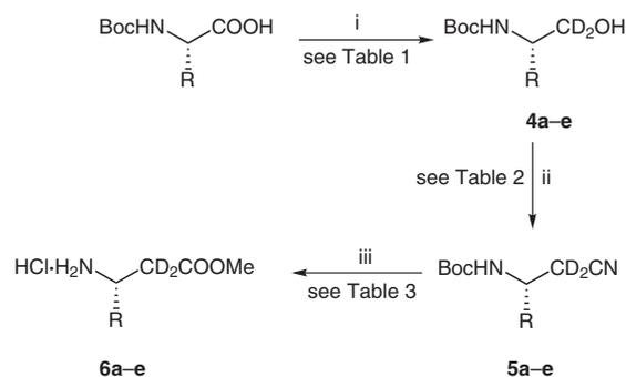
i) NMM,  $\text{MeOCOCl}$  in THF, then  $\text{NaBD}_4$  in  $\text{D}_2\text{O}$ ; ii)  $\text{PPh}_2$ ,  $\text{I}_2$ ,  $\text{HI}$  in  $\text{CH}_2\text{Cl}_2$ , then  $\text{Et}_4\text{N}^+\text{CN}^-$  in  $\text{CH}_2\text{Cl}_2$ ; iii)  $\text{HCl}$  in  $\text{MeOH}$
