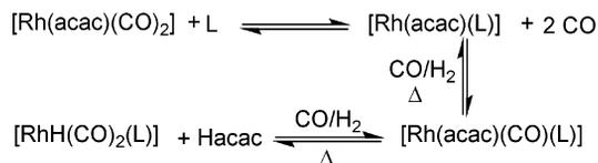
Scheme 7. Formation of  $[\text{RhH}(\text{CO})_2(\text{L})]$  from  $[\text{Rh}(\text{acac})(\text{CO})_2]$  and diphosphites (L = **1b**, **8a**).
