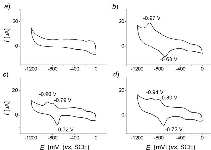
Fig. 3. Cyclic voltammograms of  $H_2TPP$  (a) and the diselenide-linked porphyrin dimers **4a–4c** (b–d, resp.) adsorbed on MWCNT-modified gold electrode in  $0.1$  M phosphate buffer solution (pH 7.4) measured at a scan rate of  $100$  mV/s
