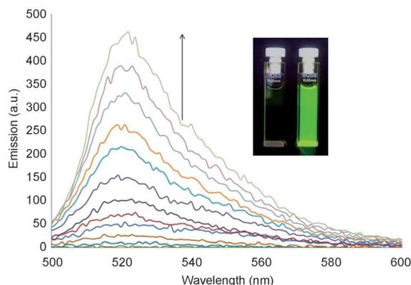
**Figure 2.** Fluorescence spectra of complex 1-Cu<sup>II</sup> (water/acetonitrile 9:1 v/v,  $1.0 \times 10^{-5}$  M) in the presence of increasing NO concentrations from 0 to 80 ppm after 5 min. Inset: the visual changes ( $\lambda_{\text{exc}} = 254$  nm) observed for 1-Cu<sup>II</sup> before and after exposure to 1 ppm of NO.
