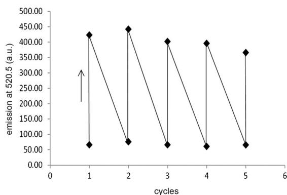
**Figure 3.** The cycles of emission intensity of 1-Cu<sup>II</sup> ( $1.0 \times 10^{-5}$  M in acetonitrile) at  $\lambda_{\text{em}} = 520.5$  nm ( $\lambda_{\text{exc}} = 500.5$  nm) upon successive exposures to NO (5 min) and to a NO-free air atmosphere (24 h).
