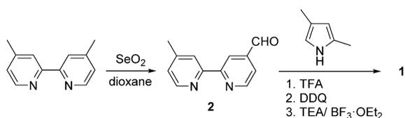
Scheme 2. Synthesis of ligand **1**. DDQ = 2,3-dichloro-5,6-dicyano-1,4-benzoquinone; TEA = triethylamine.
