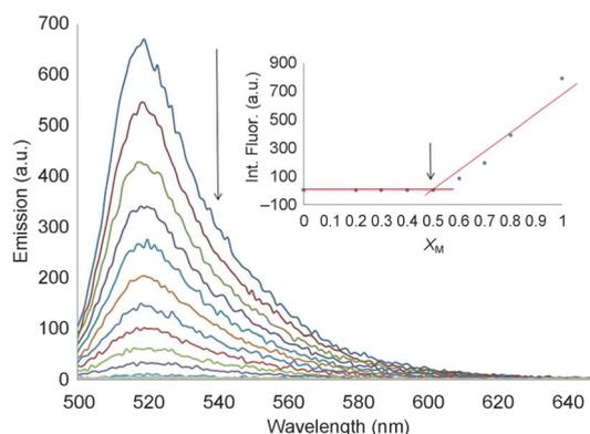
Figure 1. Fluorescence spectra of **1** (acetonitrile,  $1.0 \times 10^{-5}$  M) with increasing amounts of  $\text{Cu}^{\text{II}}$ . Inset: molar ratio graphic.
