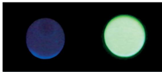
**Figure 4.** Emission of a polyethylene oxide membrane of 1-Cu<sup>II</sup> ( $\lambda_{\text{exc}} = 254$  nm) (left) and after exposure to 1 ppm of NO in air for 5 min (right).
