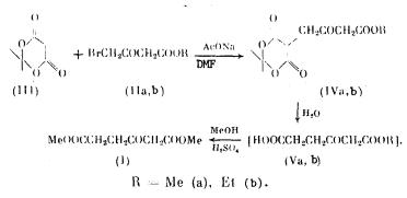
By the reaction of (III) with (IIa, b) in DMF in the presence of  $AcONa \cdot 3H_20$  we obtained the respective monoalkylation products (IVa, b); these were then cleaved according to [4] to form (Va, b), the monoesters of  $\beta$ -oxoadipic acid. Methanolysis of (Va) and (Vb) by a MeOH-H<sub>2</sub>SO<sub>4</sub> mixture gave the desired diester (I) in an overall yield of 30% based on (IIa, b).
