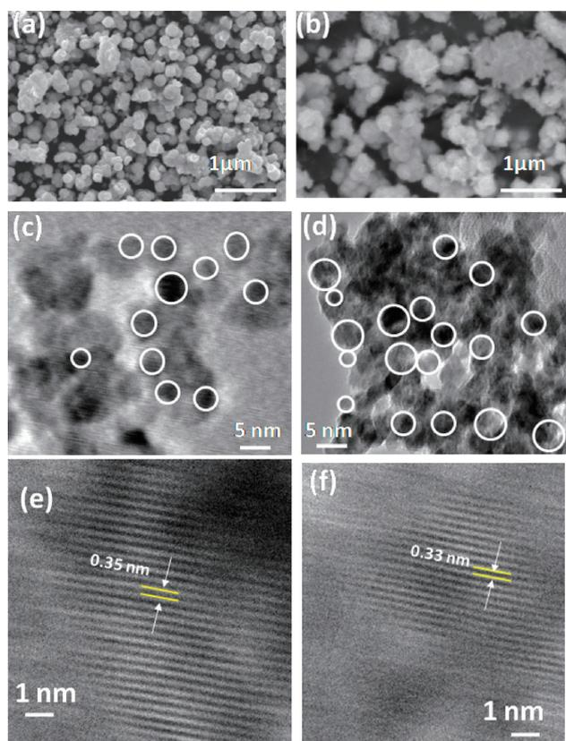
**Figure 2.** (a), (b) SEM, (c), (d) TEM, and (e), (f) HRTEM images of ZnS and CdS nanoparticles respectively.
