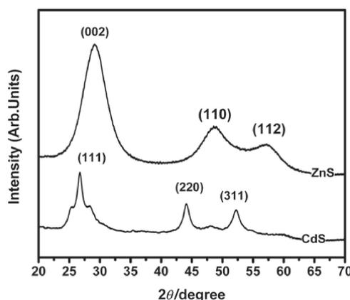
Figure 1. XRD patterns for ZnS and CdS nanoparticles.
