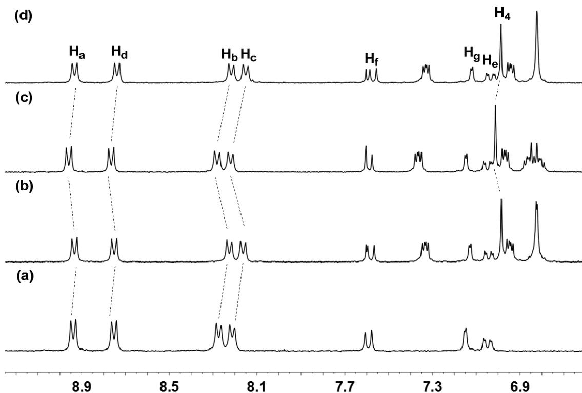
**Figure S27.** Partial  $^1H$  NMR spectra ( $CD_3CN$ , 300 MHz) of (a) free guest **3**, (b) **1** and 1.0 equiv. of **3**, (c) to the solution of b was added 4.0 equiv. of  $KPF_6$ , and (d) to the solution of c was added 6.0 equiv. of [18]-crown-6,  $[1]_0 = 2.0$  mM.
