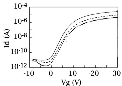
FIG. 1. Transfer characteristics measured at  $V_{\text{ds}}=0.2 \text{ V}$  for different channel lengths: continuous line  $L=5 \mu\text{m}$  dashed line  $L=20 \mu\text{m}$ , and dotted line  $L=40 \mu\text{m}$ .
