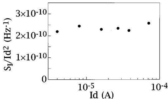
FIG. 3. Normalized drain current spectral density,  $S_I/I_d^2$ , at 20 Hz vs the mean value of the drain current  $I_d$ , for a TFT operating in the linear regime with  $L = 10 \mu\text{m}$  and  $V_g = 14 \text{ V}$ .
