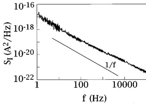
FIG. 2. Drain current spectral density for a TFT with channel length  $L = 10 \mu\text{m}$   $V_{\text{ds}} = 2 \text{ V}$  and  $V_g = 14 \text{ V}$ .
