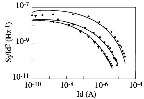
FIG. 4. Normalized drain current spectral density,  $S_I/I_d^2$ , at 20 Hz vs the mean value of the drain current  $I_d$ , for TFTs with channel length  $L = 5 \mu\text{m}$  ( $\bullet$ ),  $L = 20 \mu\text{m}$  ( $\blacksquare$ ), and  $40 \mu\text{m}$  ( $\blacktriangle$ ). Continuous lines are the best fit to Eq. (1).
