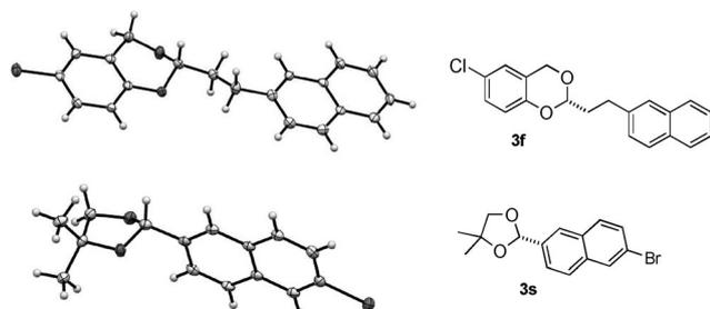
**Figure 1.** Crystal structures of acetals **3f** and **3s** (ellipsoids at the 50% probability level).<sup>[14]</sup>
