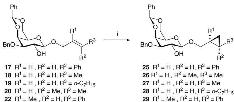
**Scheme 5.** Reagents: (i) CH<sub>2</sub>I<sub>2</sub>/ZnEt<sub>2</sub>/PhCH<sub>3</sub>.
