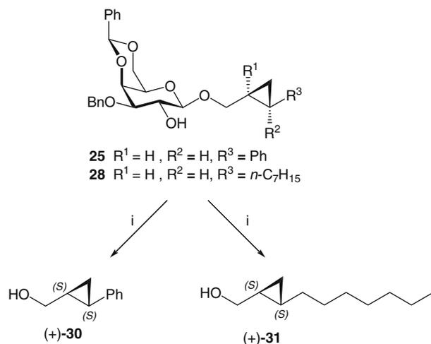
**Scheme 6.** Reagents and conditions: (i) (1) Tf<sub>2</sub>O/Py (95%); (2) DMF/Py/H<sub>2</sub>O/160 °C.
