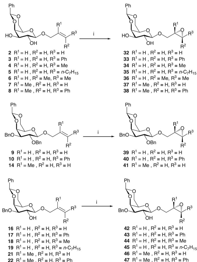
Scheme 7. Reagents and conditions: (i) *m*-CPBA/CHCl<sub>3</sub>/–15 °C.
