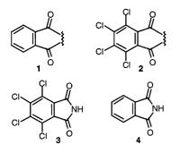
The four electron-withdrawing chlorine atoms on the aromatic ring not only faciliate nucleophilic attack at the imide carbonyls, but should also enhance the acidity of the imidic hydrogen. Thus tetrachlorophthalimide (TCP-NH) **3** should be more effective than unsubstituted phthalimide (Pht-NH) **4** in Mitsunobu reactions. In this manuscript we report our work on this problem.
