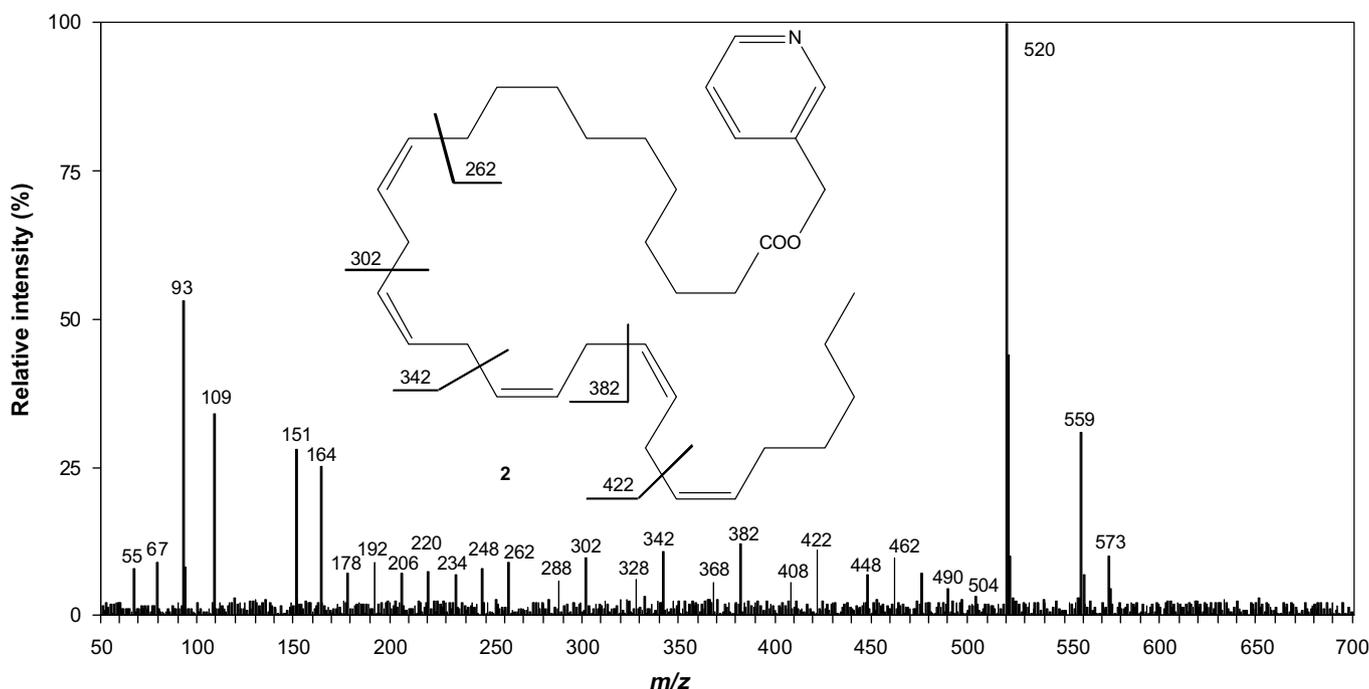
Fig. 4. Mass spectrum of picolinyl ester of 29:5n-6 acid. For explanation of values see the text.
