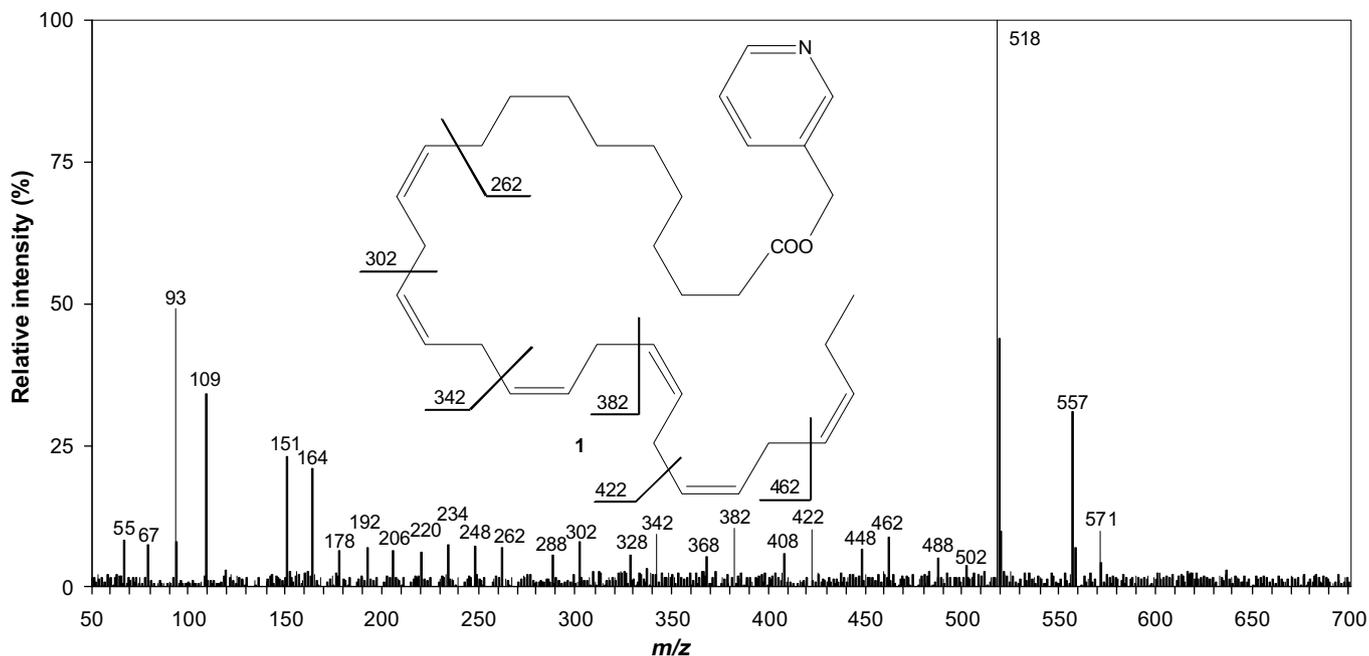
Fig. 3. Mass spectrum of picolinyl ester of 29:6n-3 acid. For explanation of values see the text.
