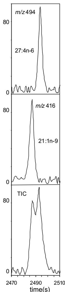
Fig. 2. LC-MS/APCI SIM and TIC chromatograms of total FAMES from *A. carterae*. Only compounds with retention times between 2470 s and 2510 s are shown.
