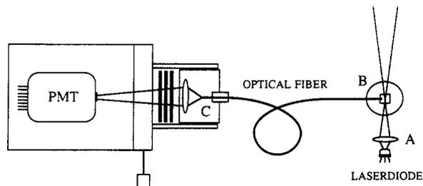
Figure 3. Light path in DIO-LIF detection system: (A) excitation light from diode laser to flow cell; (B) collection of emission light with optical fiber; (C) focussing of collected light on photomultiplier tube (PMT).
