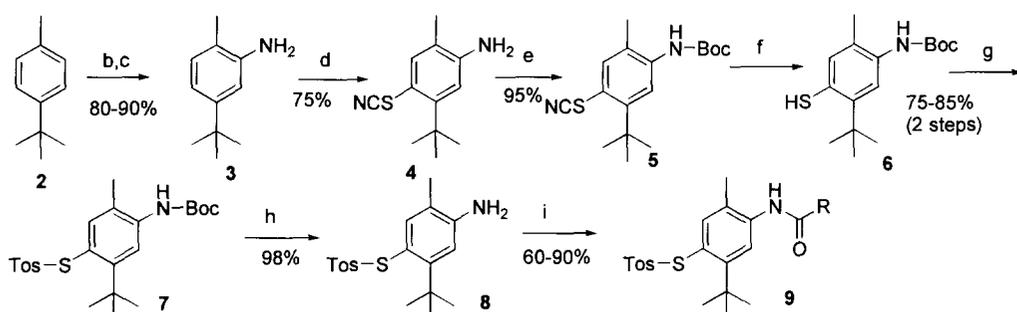
(a) anhyd  $K_2CO_3$ , 6,6'-disubstituted-2-one, DMF; (b)  $HNO_3$ ,  $H_2SO_4$ ; (c) 20% Pd/C, hydrogen (d) NaSCN, NaBr, bromine; (e)  $(Boc)_2O$ , 1 N NaOH; (f) DTT, ethanol, 0.02 M  $KH_2PO_4$  buffer; (g) Tosyl bromide,  $Et_3N$ ; (h) 4 N HCl, dioxane; (i) acid chloride,  $Et_3N$ .
