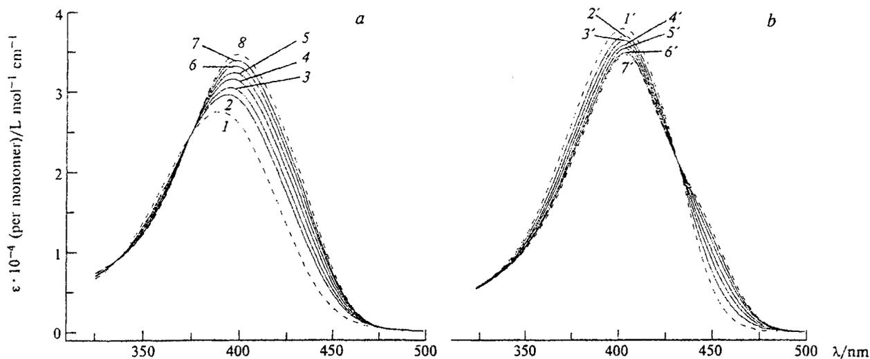
Fig. 1. Absorption spectra of complexes  $(trans-2a) \cdot Mg^{2+}$  (a) and  $(trans-2b) \cdot Mg^{2+}$  (b) in MeCN at various concentrations of the dyes:  $C_L \cdot 10^5 / \text{mol L}^{-1} = 0.08$  (2), 0.16 (3), 0.4 (4), 0.93 (5), 2.9 (6), 9.2 (7) (*trans-2a*); 0.08 (2'), 0.23 (3'), 0.73 (4'), 2.4 (5'), 9.0 (6') (*trans-2b*). Dashed curves correspond to the simulated spectra of monomeric (1, 1') and dimeric (8, 7') complexes.
