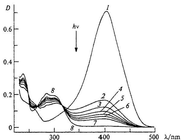
Fig. 4. Spectral changes following the photolysis of CSD *trans*-2b in MeCN ( $C_L = 2.0 \cdot 10^{-5}$  mol L<sup>-1</sup>,  $l = 1$  cm) in the presence of Mg(ClO<sub>4</sub>)<sub>2</sub> ( $C_M = 1.2 \cdot 10^{-4}$  mol L<sup>-1</sup>) by light with  $\lambda = 365$  nm and with intensity  $I = 2.8 \cdot 10^{15}$  cm<sup>-2</sup> s<sup>-1</sup>. Duration of the irradiation/min = 0 (1), 3 (2), 6 (3), 9 (4), 12 (5), 15 (6), 20 (7), 120 (8) (photocycloadduct [8·Mg<sub>2</sub>]<sup>4+</sup>).
