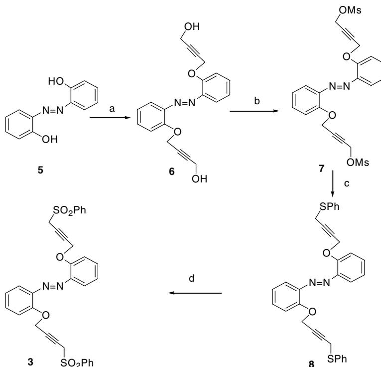
**Scheme 1.** Synthesis of bispropargyl bissulfone. Reagents and conditions: (a) 2-butyn-1,4-diol mono tosylate,  $K_2CO_3$ , DMF, rt, 12 h, 90%; (b) MsCl,  $Et_3N$ ,  $CH_2Cl_2$ , 0 °C, 15 min, 95%; (c) PhSH,  $Et_3N$ ,  $CH_2Cl_2$ , 0 °C, 30 min, 20%; (d) *m*-CPBA,  $CH_2Cl_2$ , 0 °C, 1.5 h, 90%.
