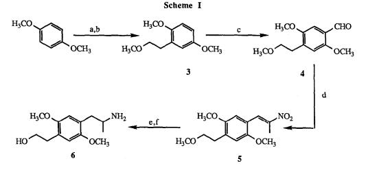
a. n-BuLi; ethylene oxide, 63%. b. NaH; CH<sub>3</sub>I, 88%. c. POCl<sub>3</sub>, HCON(CH<sub>3</sub>)C<sub>6</sub>H<sub>5</sub>, 24%. d. NH<sub>4</sub>OAc, CH<sub>3</sub>CH<sub>2</sub>NO<sub>2</sub>, 70%. e. AlH<sub>3</sub>, 93%. f. TMSCl, TMSI, 57%.
