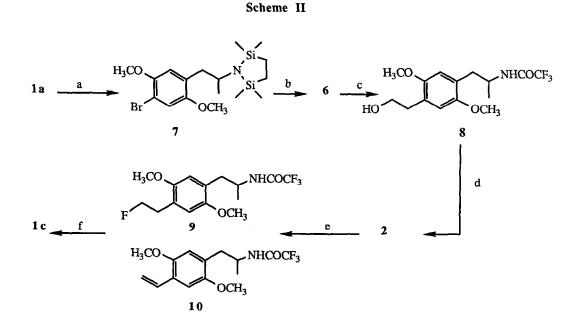
a. [ClSi(CH<sub>3</sub>)<sub>2</sub>CH<sub>2</sub>]<sub>2</sub>, 85%. b. t-BuLi; ethylene oxide; KOH, 75%. c. (CF<sub>3</sub>CO)<sub>2</sub>O; NaHCO<sub>3</sub>, 89%. d. TsCl, 96%. e. TBAF, 55%. f. KOH, 86%.
