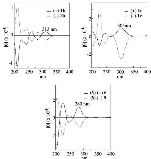
Figure 4. CD spectra of optically active telluroxides (+)-**1b**, (–)-**1b**, (+)-**1c**, and (–)-**1c** and selenoxides (*R*)-(+)-**5** and (*S*)-(–)-**5** in acetonitrile.
