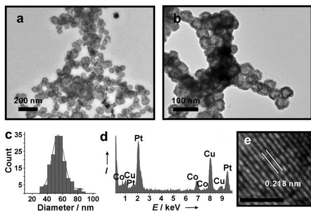
**Figure 1.** a, b) TEM images of hollow spherical CoPt nanoparticle superstructures. c) Diameter distribution of CoPt nanoparticle superstructures ( $53.9 \pm 7.9$  nm; based on 158 counts). d) EDS data for CoPt nanoparticle superstructures (Cu is from the TEM grid). e) HRTEM of a single CoPt nanoparticle showing the lattice fringes (scale bar: 2 nm).
