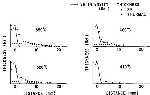
FIG. 4. Thickness profiles of the epitaxial film in the lower temperature region (surface reaction is rate-limiting). Opened circles correspond to SR-irradiated growth and closed ones to thermal growth. The thickness is normalized with the maximum thickness value of SR-irradiated growth at each temperature. Distribution of SR intensity is also presented as a solid curve.
