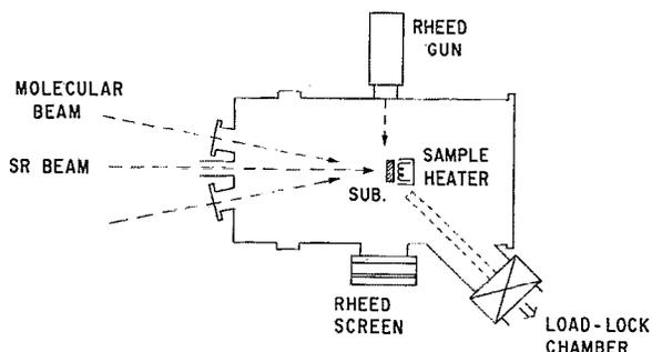
FIG. 1. SR-excited gas source MBE system.
