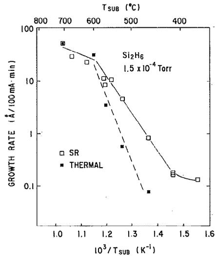
FIG. 3. Substrate temperature dependence of epitaxial growth.  $\text{Si}_2\text{H}_6$  pressure was  $1.5 \times 10^{-4}$  Torr. Opened squares correspond to SR-irradiated growth and closed ones to thermal growth.
