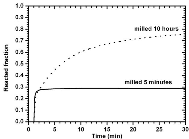
Fig. 5. Hydrogen released during hydrolysis of  $\text{MgH}_2$ -20.3 mol%  $\text{CaH}_2$  nanocomposite ball-milled for 5 min and 10 h.
