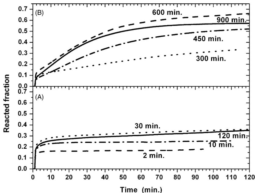
Fig. 3. Hydrogen released during hydrolysis of  $\text{MgH}_2$ -8.9 mol% Ca nanocomposite ball-milled for various durations.
