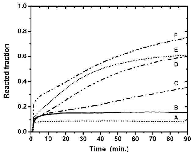
Fig. 1. Hydrogen released during hydrolysis of (A) polycrystalline  $\text{MgH}_2$ , (B)  $\text{MgH}_2$  milled 10 h,  $\text{MgH}_2$ - $X$  mol% Ca nanocomposite milled 10 h with (C)  $X = 4.7$  mol%, (D)  $X = 8.9$  mol%, (E)  $X = 20.3$  mol%, and (F) pre-milled  $\text{MgH}_2$ -20.3 mol% Ca milled 10 h.
