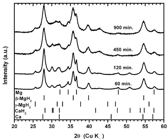
Fig. 4. X-ray powder diffraction patterns of  $\text{MgH}_2$ -8.9 mol% Ca ball-milled for different milling times.
