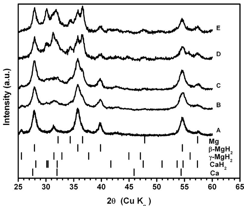
Fig. 2. X-ray powder diffraction patterns of MgH<sub>2</sub>–X mol% Ca nanocomposite milled 10 h with (A) X = 0.0 mol%, (B) X = 4.7 mol%, (C) X = 8.9 mol%, (D) X = 20.3 mol%, and (E) pre-milled MgH<sub>2</sub>–20.3 mol% Ca milled 10 h.
