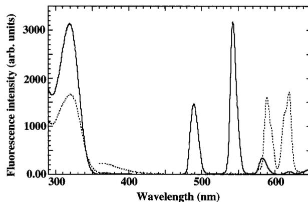
Figure 2. Excitation and emission spectra of BPTA–Tb<sup>3+</sup> (1 μM, —) and BPTA–Eu<sup>3+</sup> (20 μM, - - -) in 0.05 M borate buffer, pH 9.1.
