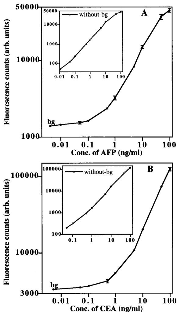
Figure 6. Calibration curves of the simultaneous measurement of AFP (A) and CEA (B) using BHHCT-Eu<sup>3+</sup>-labeled anti-AFP antibody, biotinylated anti-CEA antibody, and BPTA-Tb<sup>3+</sup>-labeled SA; bg, background. The inset curves are the plot of the background-subtracted signals vs the concentrations of AFP and CEA.
