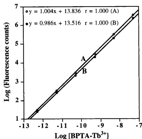
Figure 3. Log(fluorescence count) vs log[BPTA–Tb<sup>3+</sup>] in 0.05 M Tris-HCl buffer, pH 8.0: (A) free BPTA–Tb<sup>3+</sup>. (B) BPTA–Tb<sup>3+</sup> bound to SA. The concentration of BPTA–Tb<sup>3+</sup> is in molar and the fluorescence count is in arbitrary units.
