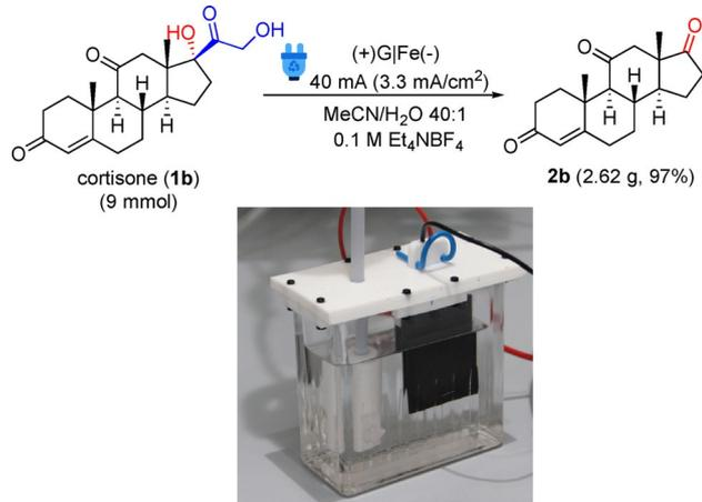
**Figure 5.** Multigram scale electrochemical synthesis of 17-ketosteroid **2b**.
