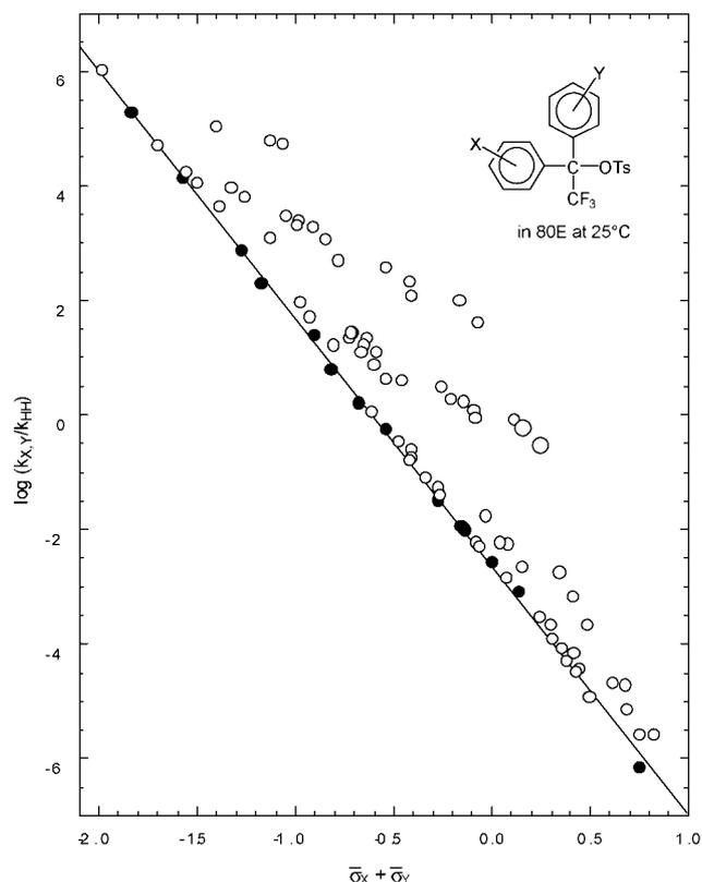
**Figure 1.** Additivity relationship against the sum of  $\bar{\sigma}$  ( $r = 1.17$ ) for substituent effects on the solvolysis of 1,1-diaryl-2,2,2-trifluoroethyl tosylates in 80% aqueous ethanol at 25 °C. Closed circles are for the symmetrical  $X = Y$  subseries **1**
