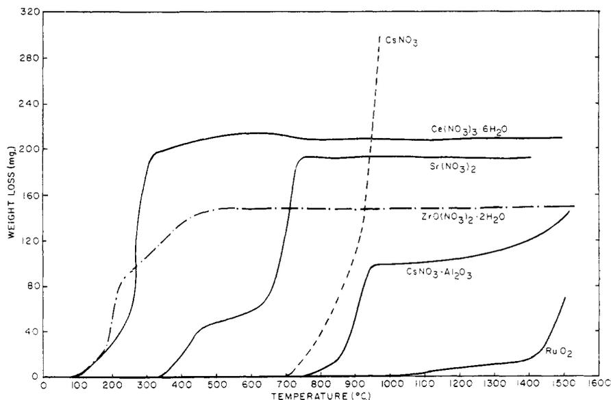
Figure 2. TGA of fission product oxides and nitrates
