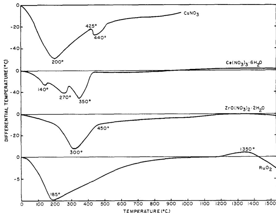
Figure 1. Thermograms of fission product oxides and nitrates
