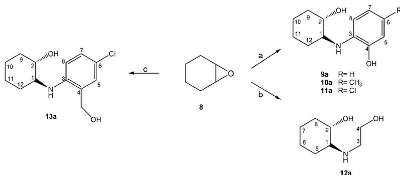
**Scheme 3.** (a) 2-Aminophenol, 2-amino-5-methylphenol, or 2-amino-5-chlorophenol, (b) ethanolamine, and (c) 2-amino-5-chlorobenzyl alcohol.
