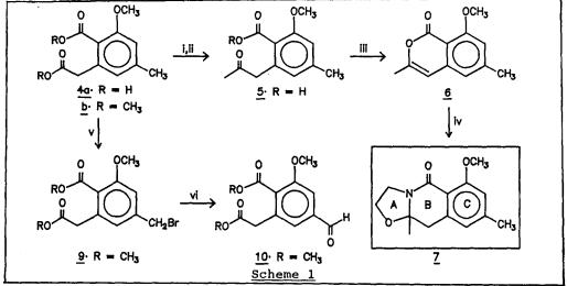
Reagents & Yield: (i) Ac20, Py., 30°C, 10h, 73%; (ii) 10% ag. NaOH, , 1h; (iii) Ac20, HClO4(Cat.), EtOAc, 30°C, 4h, 77% from 4a; (iv) 2-aminoethanol, MeOH, 30°C, 12h, 50%; (v) N-bromosuccinimide, AIBN, CCl4, , 2h, 60%; (vi) [(n-C4H9)4N]2Cr207, CHCl3, , 2h, 80%.
