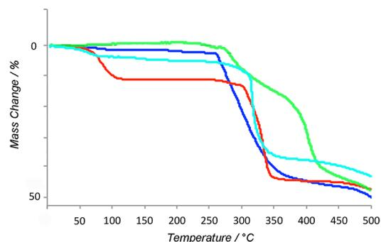
**Figure 6.** Thermogravimetric analysis curves for complexes **1a** (green), **1b** (blue), **2a** (cyan), and **2b** (red).
