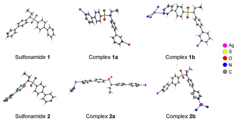
**Figure 1.** Thermal ellipsoid models of the crystal structures of the sulfonamide ligands **1** and **2**, and those of the corresponding Ag(I) complexes **1a**, **1b**, **2a**, and **2b**. The ellipsoids of all non-hydrogen atoms are drawn at the 50% probability level while isotropic hydrogen atoms are represented by spheres of arbitrary size. The counteranions and solvent molecules are omitted for clarity.
