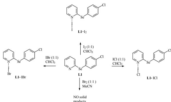
Scheme 2. Schematic representation of the compounds obtained from the reaction of **L1** with I<sub>2</sub>, Br<sub>2</sub>, ICl and IBr.
