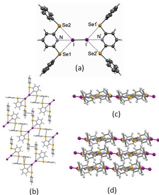
Figure 5. (a) ORTEP view of the bridging adduct unit in (**L4**)<sub>2</sub>·I<sub>2</sub>, displacement ellipsoids are drawn at the 50% probability level, I' = -x, -y, -z; (b) 2-D array of interacting (**L4**)<sub>2</sub>·I<sub>2</sub> units viewed normal to the (121) plane, and (c) along the (121) plane; (d) assembly of three instances of 2-D sheets of interacting (**L4**)<sub>2</sub>·I<sub>2</sub>.
