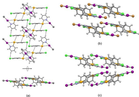
Figure 2. Crystal packing comparison for the four adducts of **L1**. (a) Common 2-D assembly viewed along two perpendicular directions. The X atom is colored as grey to represent a generic 1:1 CT adduct **L1**·IX; (b) Crystal packing of structure **L1**·IBr as representative for the set of isomorphous structures **L1**·I<sub>2</sub>, **L1**·IBr and **L1**·ICl, viewed down the [111] direction; (c) Crystal packing of structure **L2**·ICl viewed down the [110] direction.
