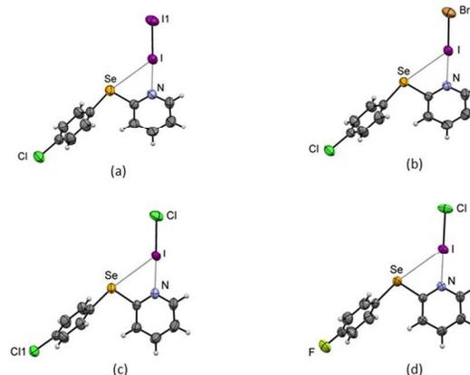
Figure 1. ORTEP view of the asymmetric unit in (a) **L1**·I<sub>2</sub>; (b) **L1**·IBr; (c) **L1**·ICl; (d) **L2**·ICl. N···I = 2.497(3), 2.410(3), 2.368(2), 2.336(3) Å; I–X = 2.7631(9), 2.6229(9), 2.5311(9), 2.511(1) Å; N–I–X = 178.17(7), 178.74(7), 178.92(6), 179.52(7)° for **L1**·I<sub>2</sub>, **L1**·IBr, **L1**·ICl and **L2**·ICl, respectively. Displacement ellipsoids are drawn at the 50% probability level.
