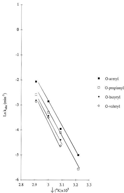
**Figure 4—Arrhenius plots of the rates of hydrolysis of aliphatic oxprenolol esters ( $\mu = 0.5$ ) at pH 5.0.**
