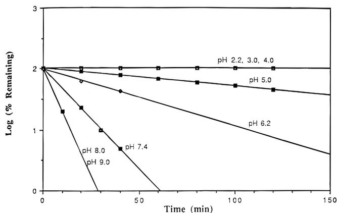
**Figure 1**—First-order plots for the degradation of *O*-acetyloxprenolol over the pH range 2.2–9.0 at 37 °C.
