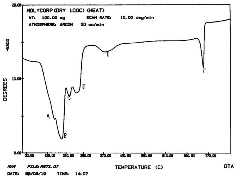
Fig. 13. DTA curve of a mixture containing primarily  $\text{NdCl}_3 \cdot 5\text{H}_2\text{O}$ .
