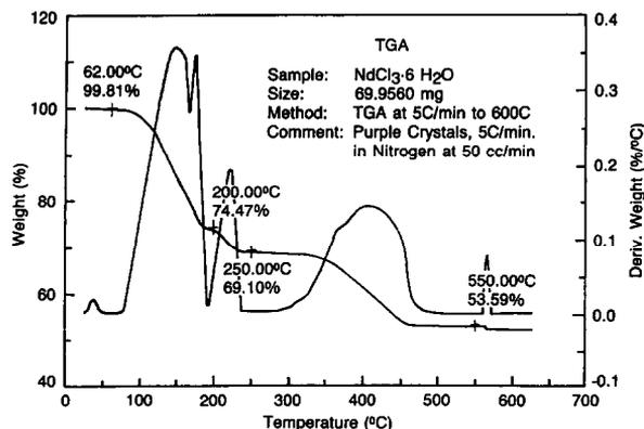
Fig. 5. TGA curve of NdCl<sub>3</sub>·6H<sub>2</sub>O.
