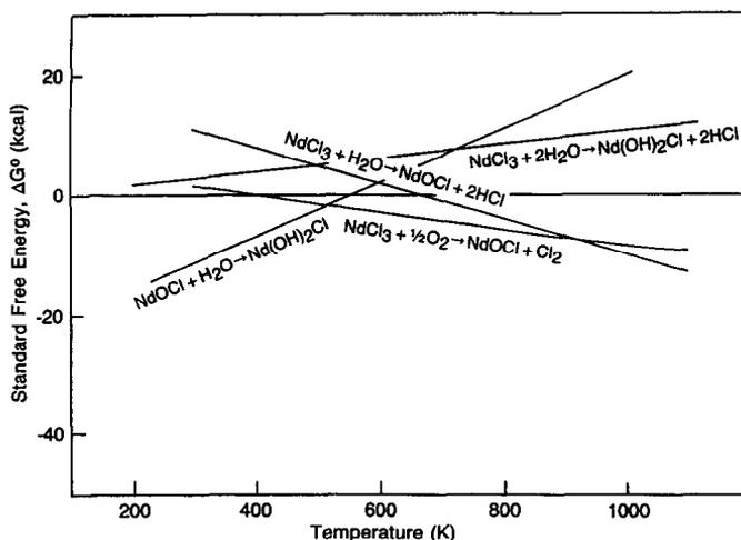
Fig. 6. Standard free energy change  $\Delta G^\circ$  of reactions relevant to dehydration vs. temperature.
