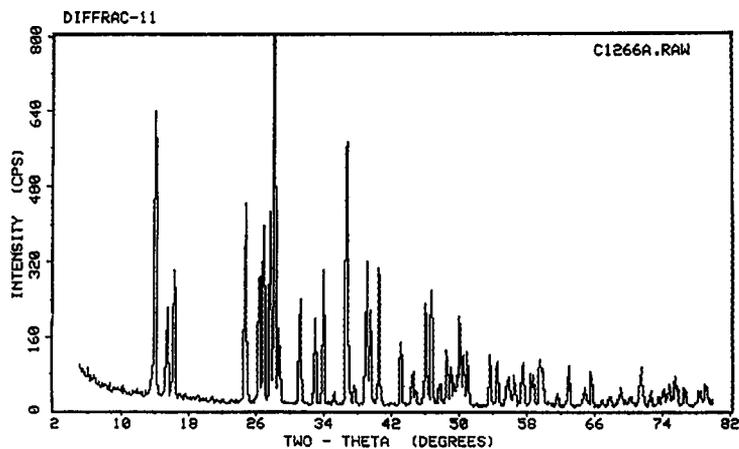
Fig. 10. XRD diffraction pattern of  $\text{Nd}(\text{OH})_2\text{Cl}$ .
