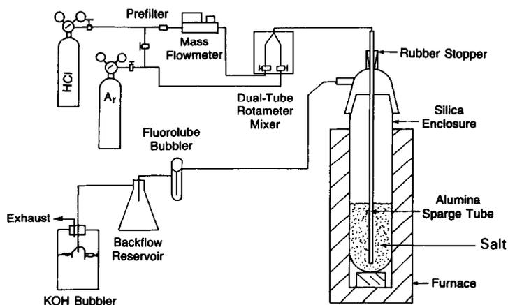
Fig. 7. Schematic diagram of the apparatus for dehydration in argon-HCl.
