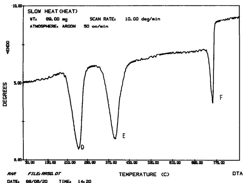
Fig. 11. DTA curve of a mixture consisting of  $\text{NdCl}_3 \cdot \text{H}_2\text{O}$ – $\text{Nd}(\text{OH})_2\text{Cl}$ – $\text{NdCl}_3$ .
