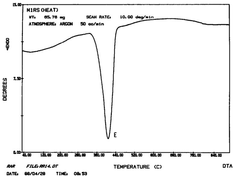
Fig. 9. DTA curve of  $\text{Nd}(\text{OH})_2\text{Cl}$ .
