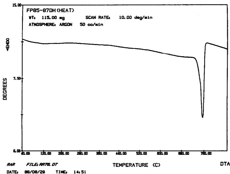
Fig. 2. DTA curve of anhydrous pure  $\text{NdCl}_3$ .
