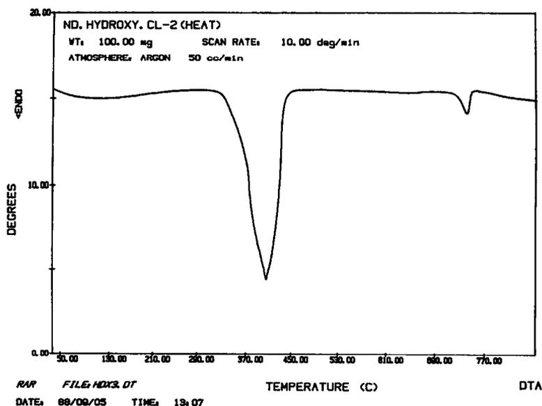
Fig. 15. DTA curve of  $\text{Nd}(\text{OH})_2\text{Cl}$  after treatment with HCl at 300 °C.
