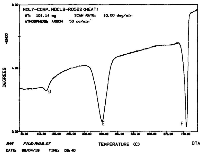
Fig. 8. DTA curve of batch 1.
