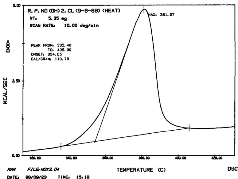
Fig. 14. DSC curve of  $\text{Nd}(\text{OH})_2\text{Cl}$ .
