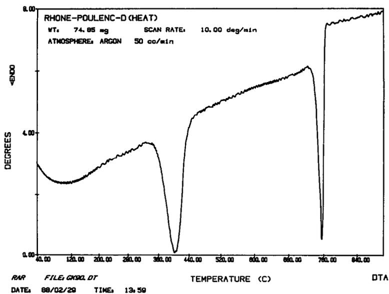
Fig. 3. DTA curve of "anhydrous"  $\text{NdCl}_3$  from Rhône-Poulenc.
