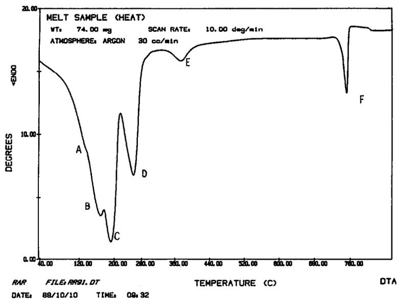
Fig. 12. DTA curve of a mixture containing predominately  $\text{NdCl}_3 \cdot 4\text{H}_2\text{O}$ .
