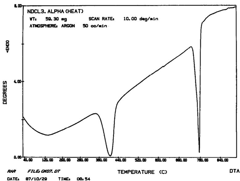
Fig. 4. DTA curve of "anhydrous"  $\text{NdCl}_3$  from ALFA.
