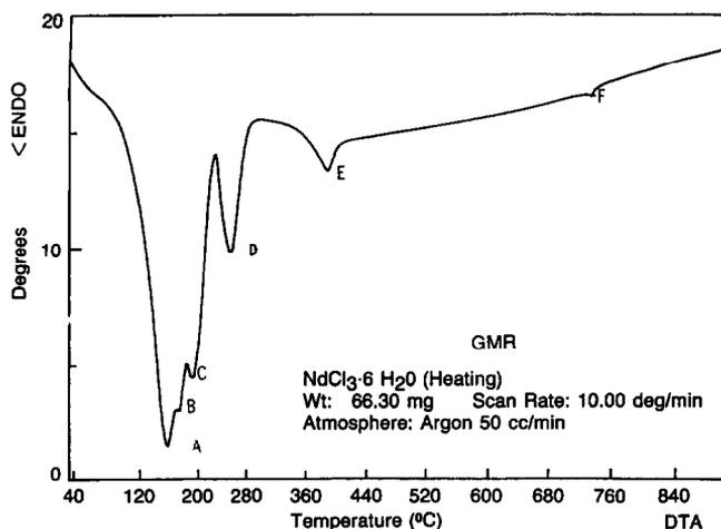
Fig. 1. DTA curve of  $\text{NdCl}_3 \cdot 6\text{H}_2\text{O}$ .
