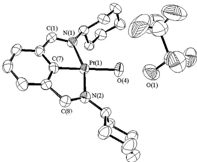
**Figure 1.** Representation of the crystal structure of **1a**. Selected bond distances (Å) and angles (deg): C(7)–Pt(1)=1.903(5), N(1)–Pt(1)=2.056(5), N(2)–Pt(1)=2.052(5), O(4)–Pt(1)=2.183(5), C(1)–N(1)=1.294(7), C(8)–N(2)=1.293(7), N(1)–Pt(1)–N(2)=159.20(18), C(7)–Pt(1)–O(4)=176.92(18).
